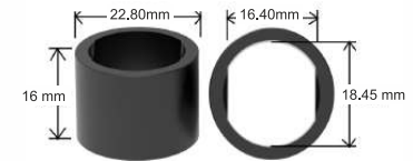
INNER BEARING T.C 8 SERIES ( D TYPE-OD-22.80 MM )
